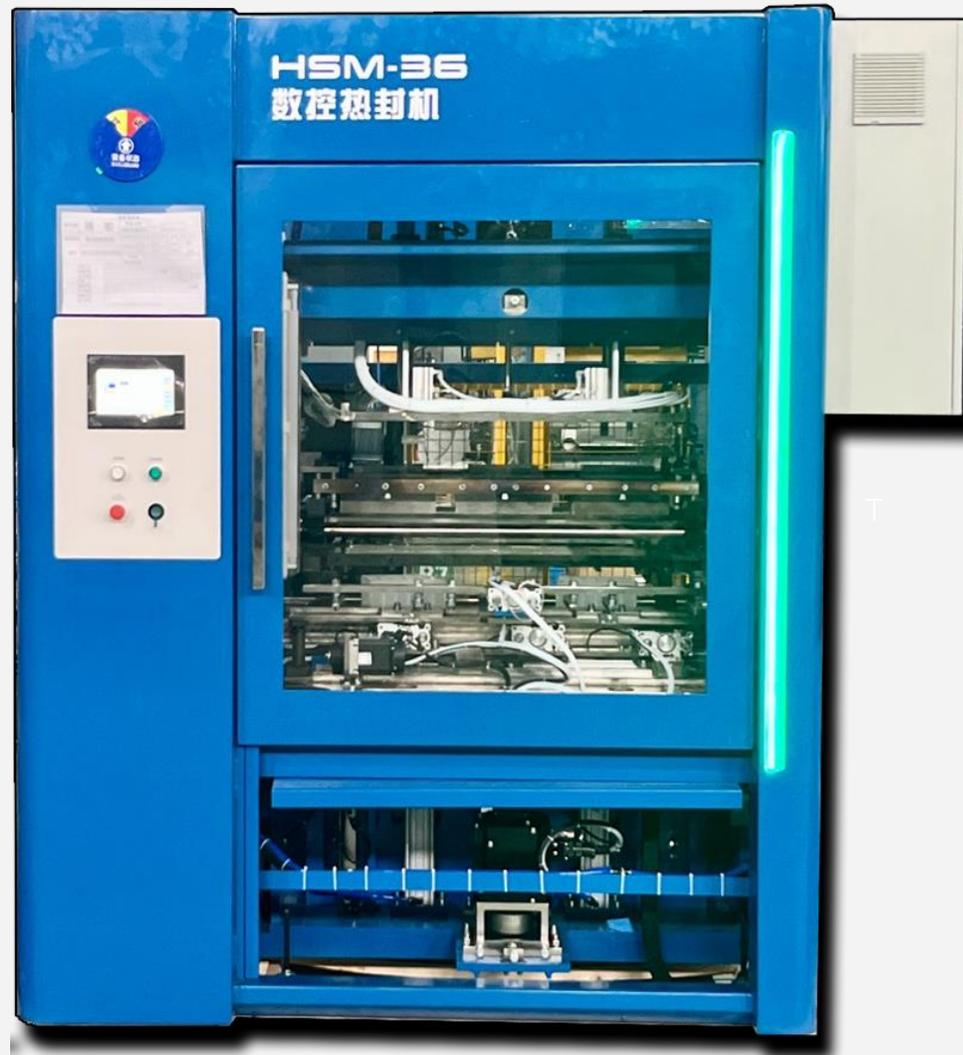
**3 batteries with 1\*6 structure can be sealed at a time**
