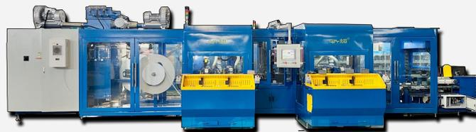
**Double Channel Envoloping and Stacking Machine**
