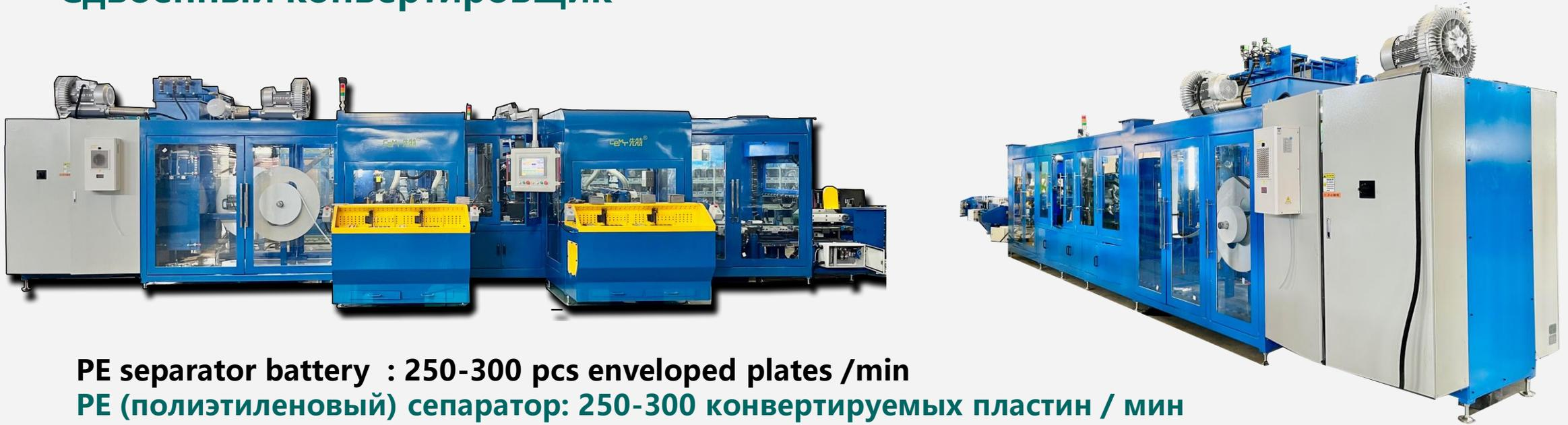
**PE separator battery : 250-300 pcs enveloped plates /min**
