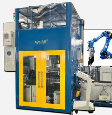
**Double Mould Cast On Strap Machine**
